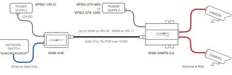
Connect 1-2 cameras or POE / non-POE devices to the RJ45 ports.
